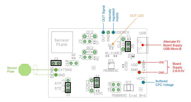
The assembly drawing illustrates the most important connection points and the initially mounted jumpers.
