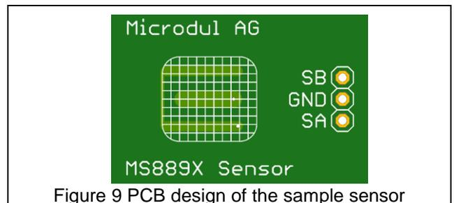
Figure 9 PCB design of the sample sensor
