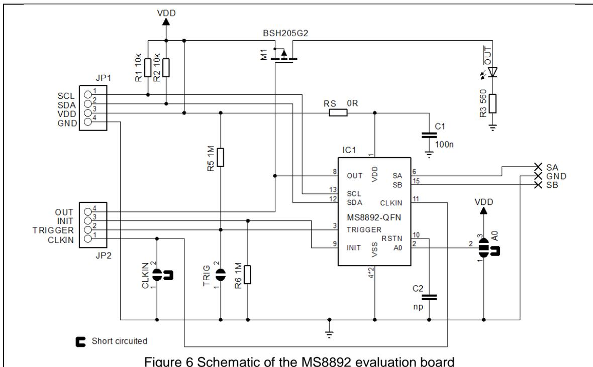
The schematic of the evaluation board is shown in Figure 6. Most of the MS8892B signals are available on three connectors JP1, JP2 and JP3. The pinning of the three connectors is given in Table 4. The I<sup>2</sup>C address input A0 is initially soldered to VSS on the backside of the evaluation board. This connection can be easily removed and soldered to VDD to enable the alternate I<sup>2</sup>C address. The pin TRIGGER is pulled to VDD level by R5. This allows to control TRIGGER from
