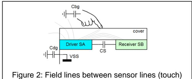
The change in capacitance between «no touch» and «touch» depends on many parameters. For example:
