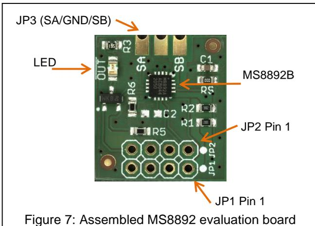
Figure 7: Assembled MS8892 evaluation board
