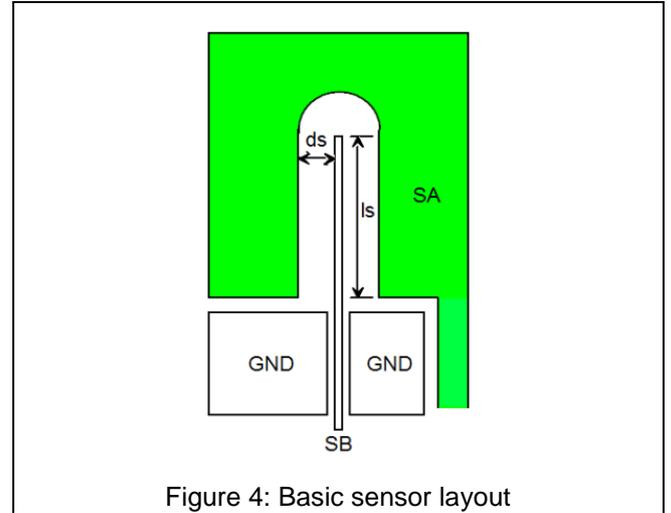
The sensor layout presented in Figure 4 is an example. Other sensor shapes can be realized. Examples of sensor dimensions and corresponding sensor capacitances based on the sensor layout presented in Figure 4 are listed in Table 2.
