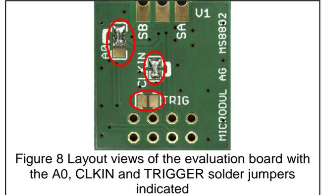
Figure 8 Layout views of the evaluation board with the A0, CLKIN and TRIGGER solder jumpers indicated
