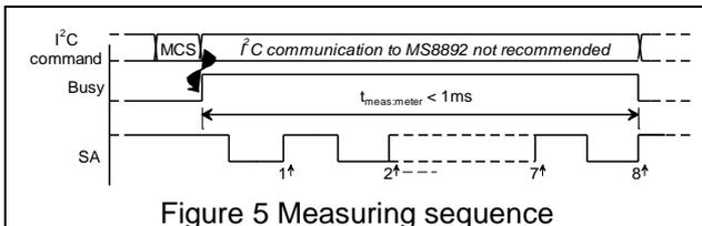
Figure 5 Measuring sequence
