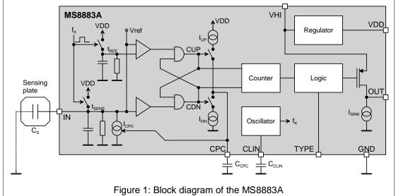
Figure 1 illustrates the functional principle of of the MS8883A.
