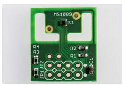
The MS1089 is a fully integrated, tested and calibrated  $I^2C$  digital temperature sensor with a typical accuracy of  $0.3^{\circ}C$  from 0 to  $60^{\circ}C$ . Its temperature range is  $-40^{\circ}C$  to  $85^{\circ}C$  with three selectable resolutions of  $0.1^{\circ}C$ ,  $0.05^{\circ}C$  and  $0.025^{\circ}C$ , and a supply range of 1.8-3.6V.
