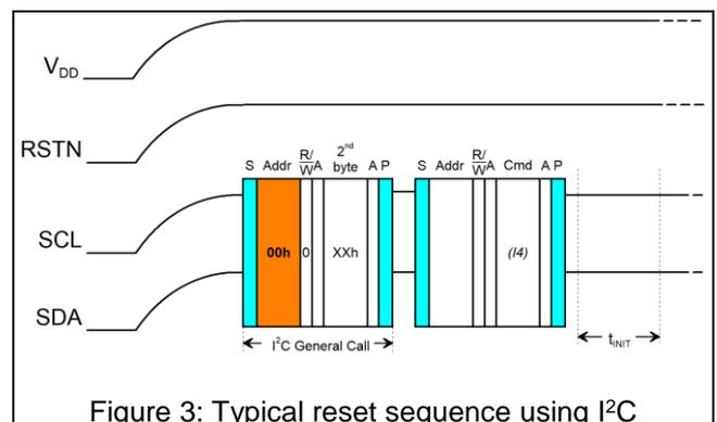
Figure 3: Typical reset sequence using I<sup>2</sup>C
