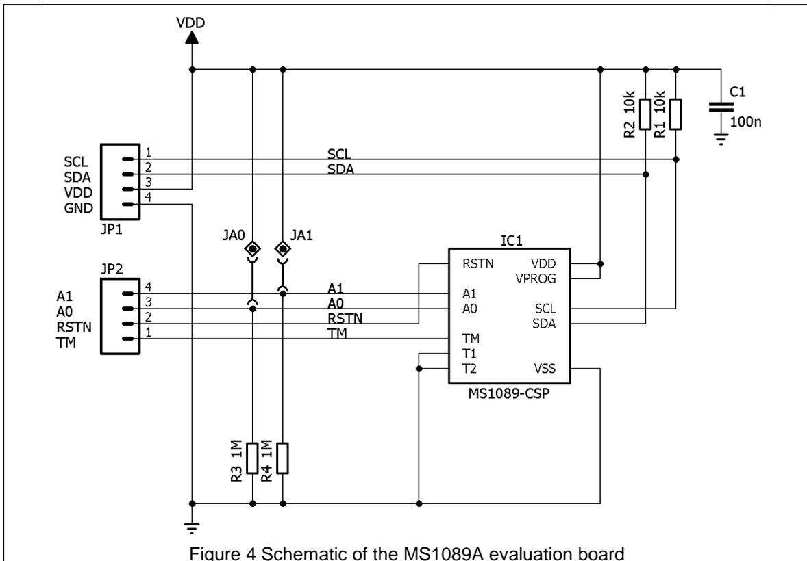
Figure 4 Schematic of the MS1089A evaluation board
