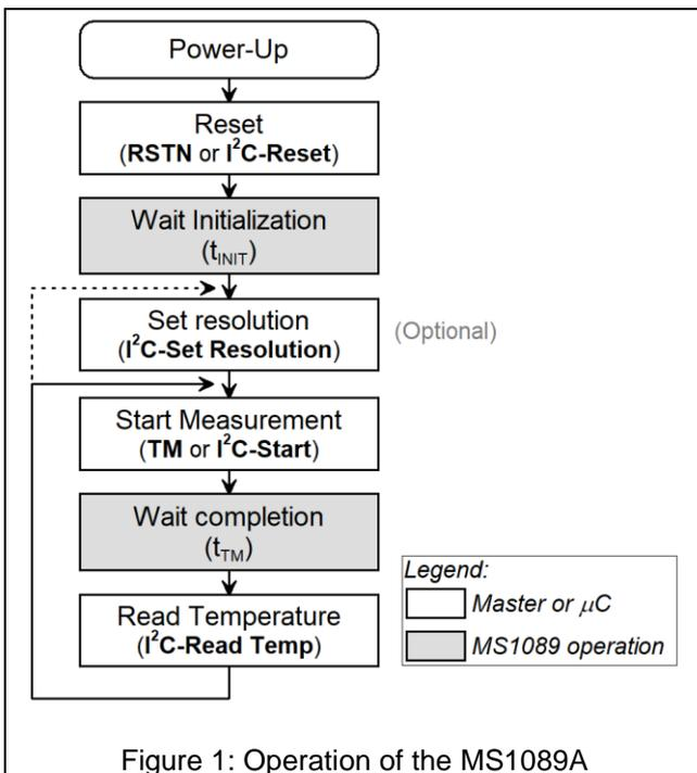
Figure 1: Operation of the MS1089A
