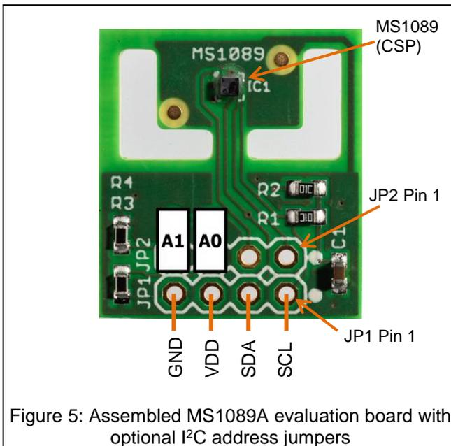
Figure 5: Assembled MS1089A evaluation board with optional I<sup>2</sup>C address jumpers
