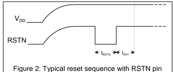
Figure 2: Typical reset sequence with RSTN pin
