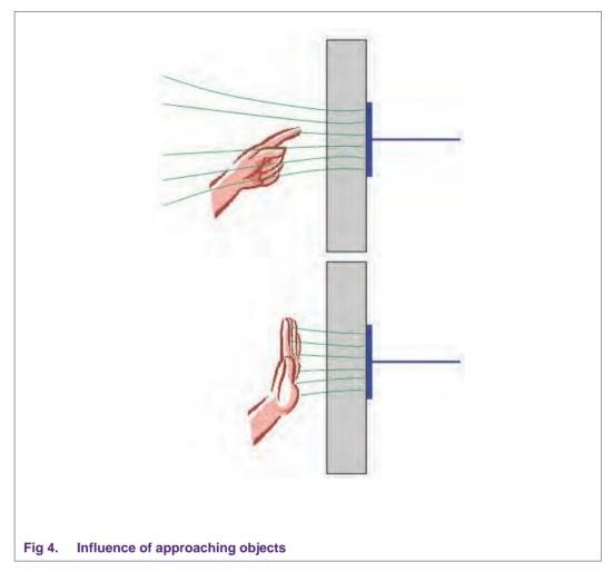
The minimal sensor area should not be smaller than the triggering object area. A larger sensing area is recommended. The sensor area or CCPC must be increased in cases when switching has to take place through different layers (e.g. over distance, with differing permittivity).
