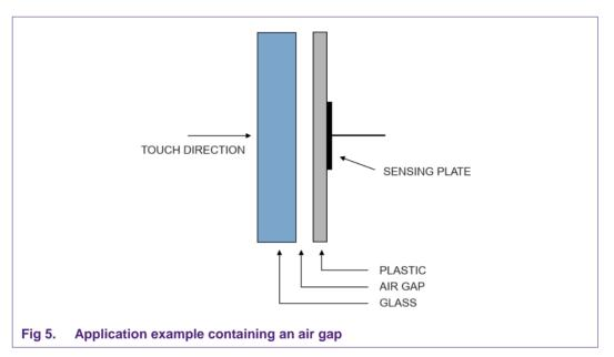
Materials having higher relative permittivity support higher sensitivity because the electrical field strength is proportional to the relative permittivity and inverse proportional to the thickness. The air gap above is an issue because the relative permittivity  $\epsilon_r = 1$  is low compared to plastic or glass.
