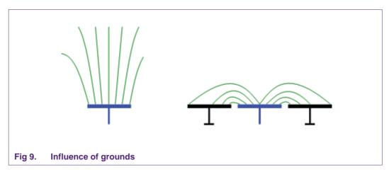
The electric field takes the shortest path to ground. As shown in <u>Figure 9</u>, the presence of the ground flattens the field and therefore shortens the switching distance and sensitivity in comparison to the example without a ground nearby.
