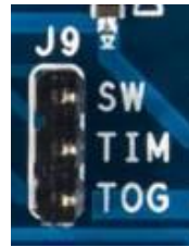
Fig 2. Selection of operating mode using jumper J9
